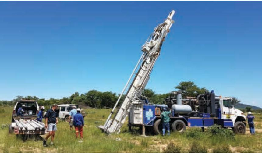
Preparing for percussion drilling at Frischgewaagt.
