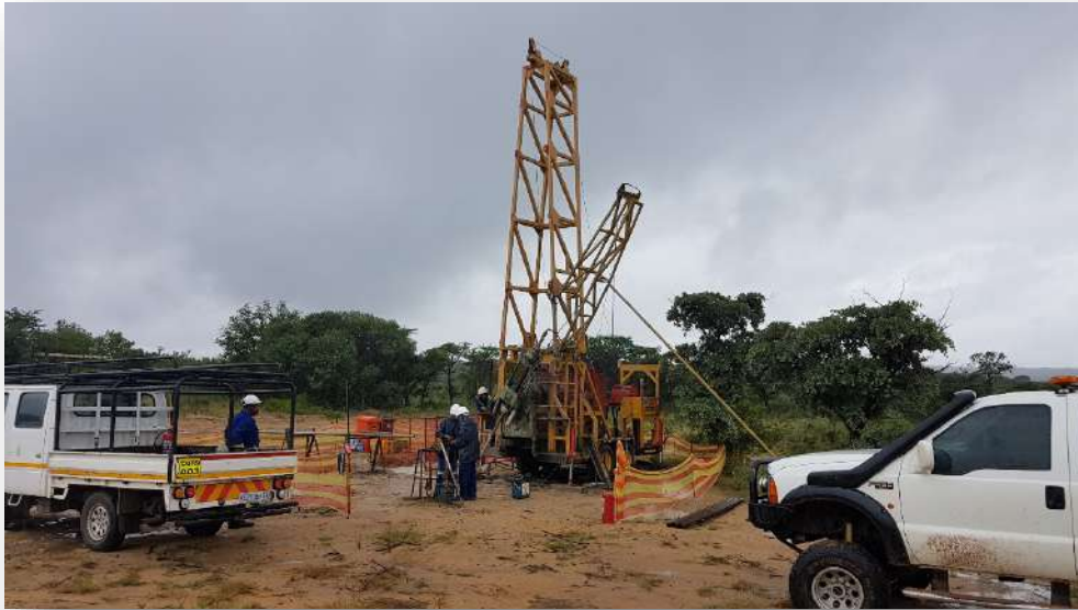
Plate 6.1 Drilling rig used by Waterman to provide NQ 47.6mm diameter core on the Thorny River project
