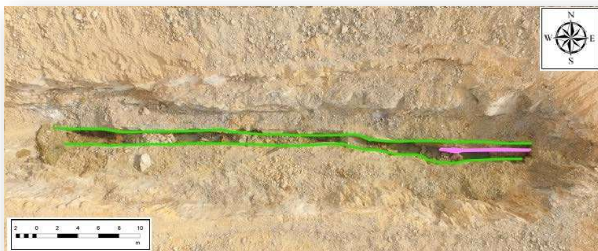
Figure 6.18 Aerial footage (from the drone) of the trench once it was fully sampled. The blow is to the west, the east shows a bifurcation (Green is kimberlite, pink is granite). Trench is 45m in strike length. The thickness of the kimberlite varied from 1-4 metres, with an average thickness of 2m
